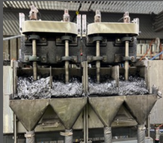
Flotation cell test work underway.
