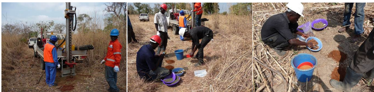
Auger drilling, sampling and logging at the South Wa soil anomaly
