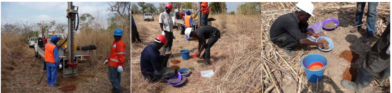
Auger drilling, sampling and logging at the South Wa soil anomaly
