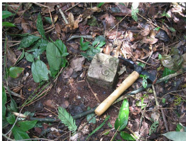
Concrete plug at Wuowuo Hill marking a drill hole from the 1970's feasibility study.
