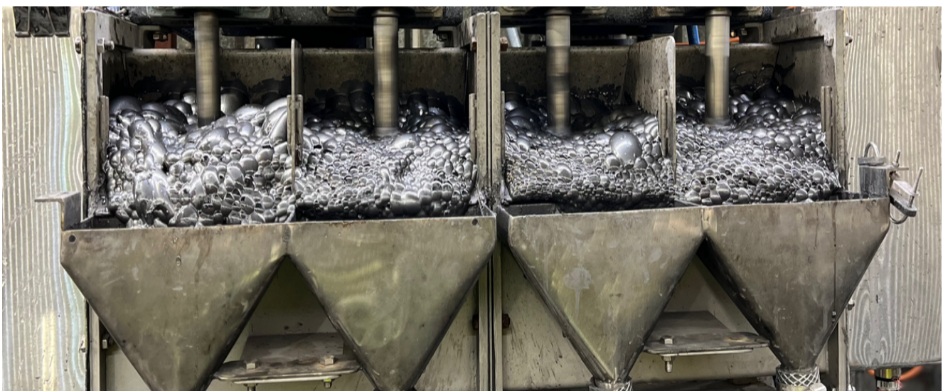
Photo 1: Flotation cells containing Kambale Graphite Project graphite concentrate
