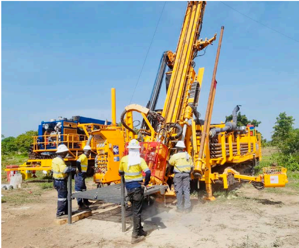
Photo 1: The first hole being collared in the Phase 3 RC drill hole programme at the Kambale Graphite Project.
