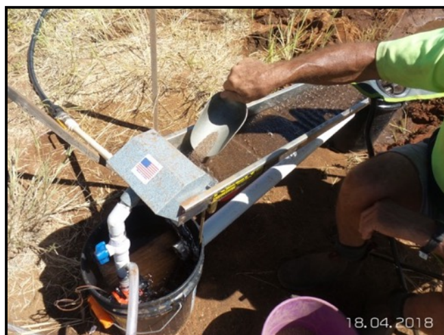
Photo 1: Feeding stream sediment sample into the field portable super-concentrator
