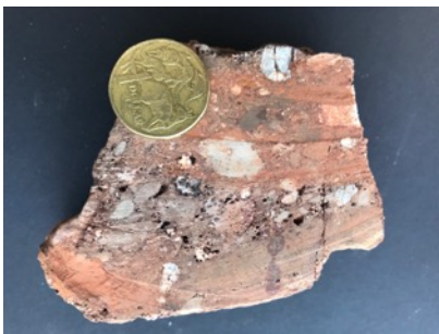
Photos 2A, 2B and 2C: Saw cut samples of conglomerate boulders retrieved from spoil heaps
