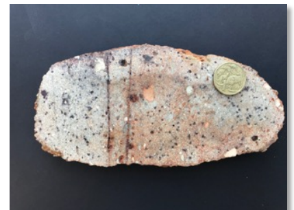
Photos 2A, 2B and 2C: Saw cut samples of conglomerate boulders retrieved from spoil heaps
