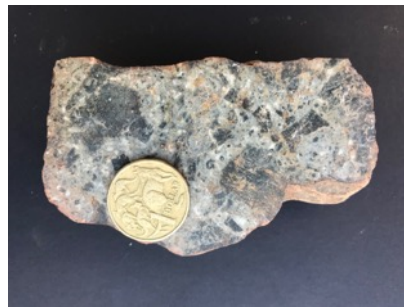
Photos 2A, 2B and 2C: Saw cut samples of conglomerate boulders retrieved from spoil heaps
