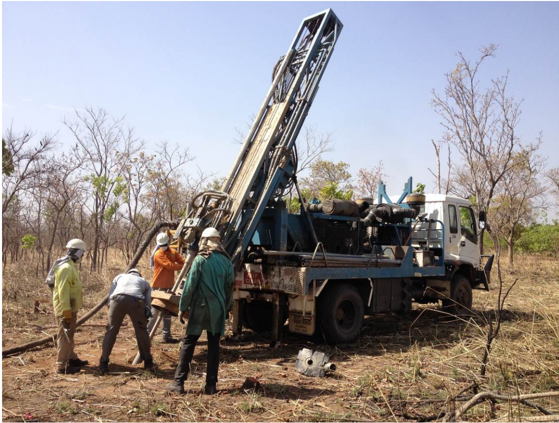
RAB Drilling at Bundi
