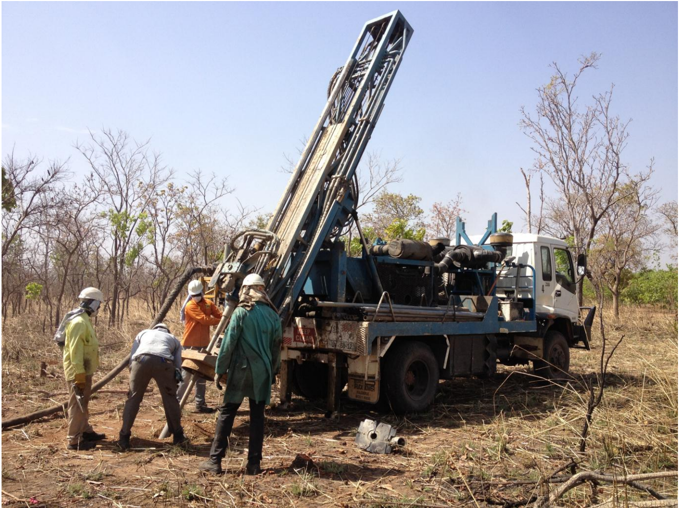
RAB drilling at Wa South – the area is largely masked by a veneer of alluvial sand and gravels
