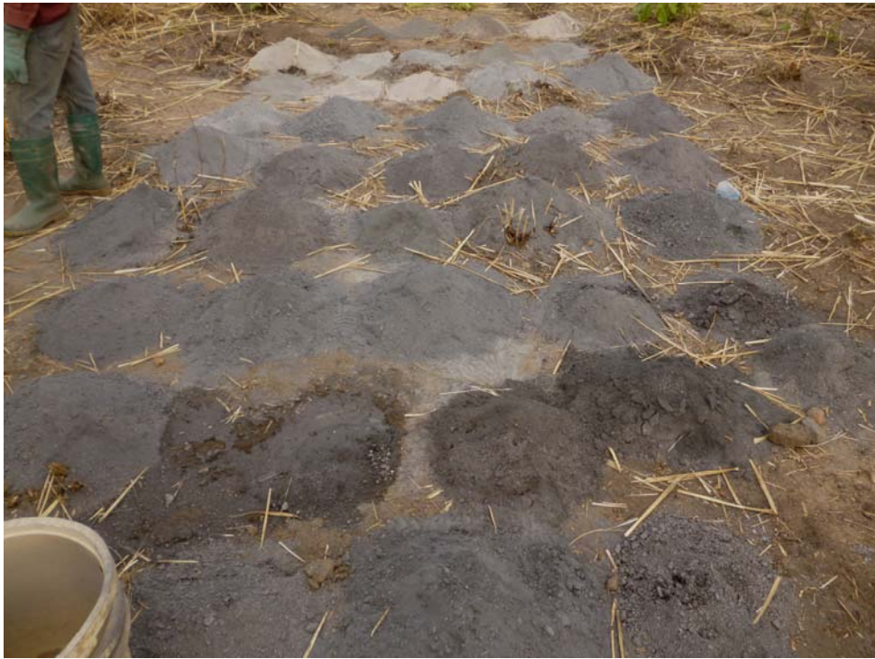
Drill cuttings from hole KBRB 12 that reported 48m @ 9.8%C from surface to EOH, including 24m @ 12.9%C from 13m.
