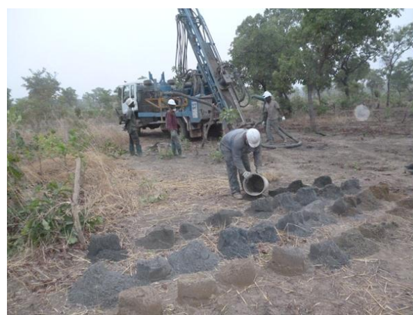
RAB drilling at hole KBRB 31 with graphitic schist from 13m down hole. The drill rig is owned by Castle Minerals.
