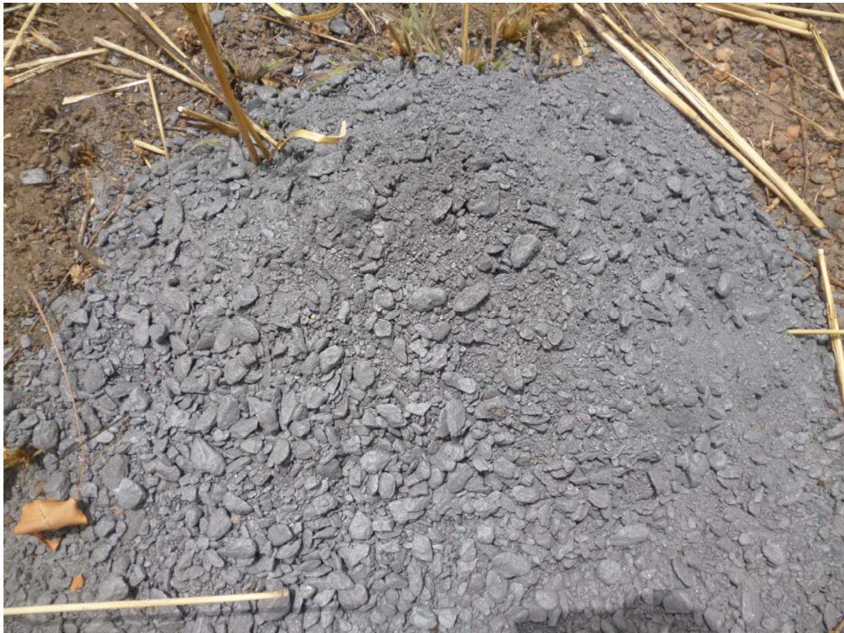
Drill sample of graphitic rich schist from hole KBRB 03
