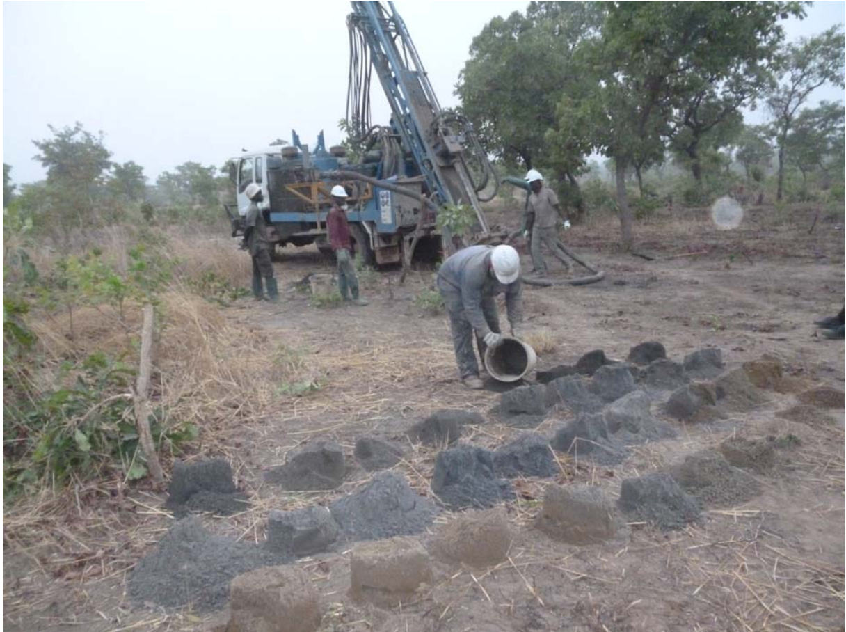
RAB drilling at hole KBRB 31 with graphitic schist from 13m down hole. The drill rig is owned by Castle Minerals.
