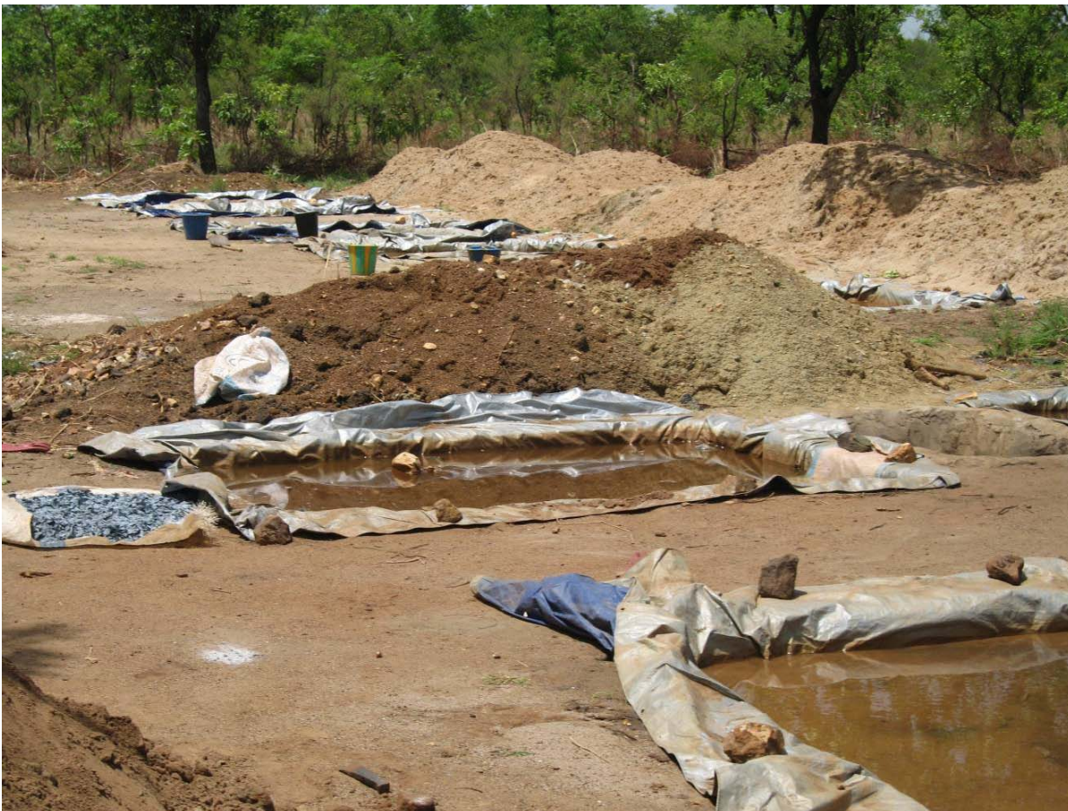
Lined vats leaching Kandia gold ore (crushed metasediment) with gold adsorbed onto zinc shavings
