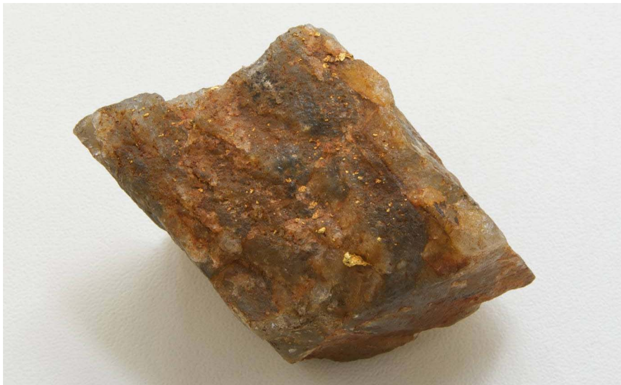
Native gold (yellow blebs) in 4cm wide quartz veinlet from Kandia artisanal workings. (This sample was not submitted for analysis)
