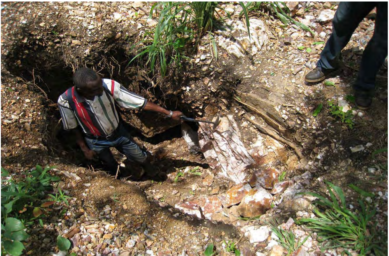
Artisanal working on a north dipping laminated vein - the vein assayed 17.07g/t gold
