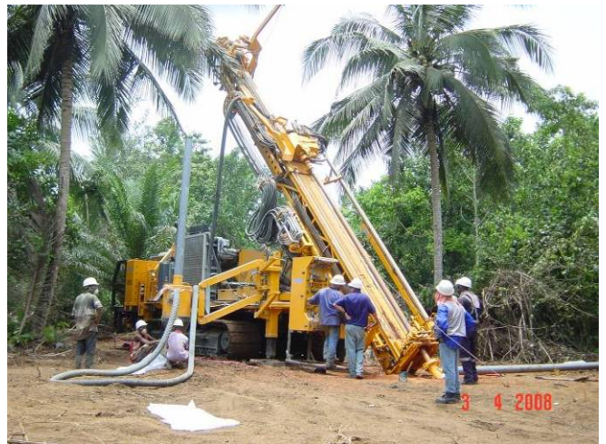
Reverse circulation drilling at Akoko North
