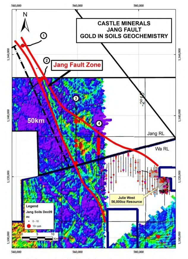
Jang Fault soil traverses (1-4) with gold geochemistry results over regional electromagnetic image
