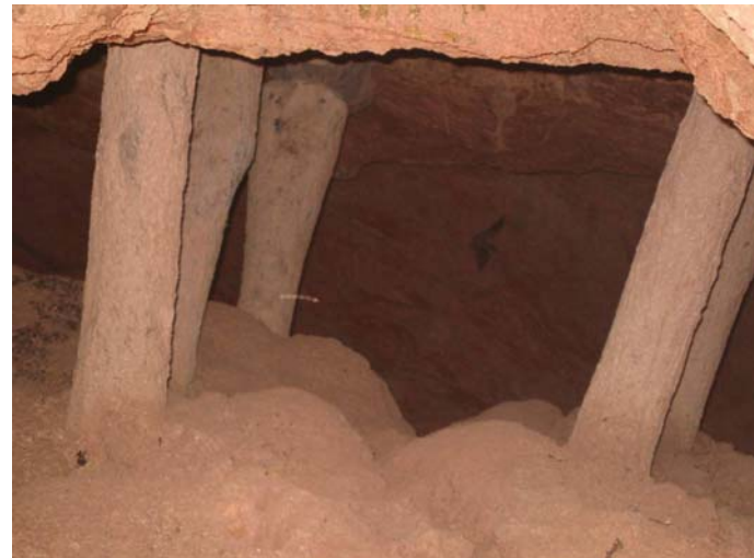
Prospecting shafts at the Charlie vein (left) and open stopes with timber supports (above) used by artisanal miners at Charlie.
