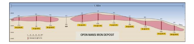
Cross section through Wuowuo Hill deposit. The Opon Mansi Iron Deposits are located along a range of hills with preliminary investigations revealing iron occurrences on top of most of the hills in the range.
